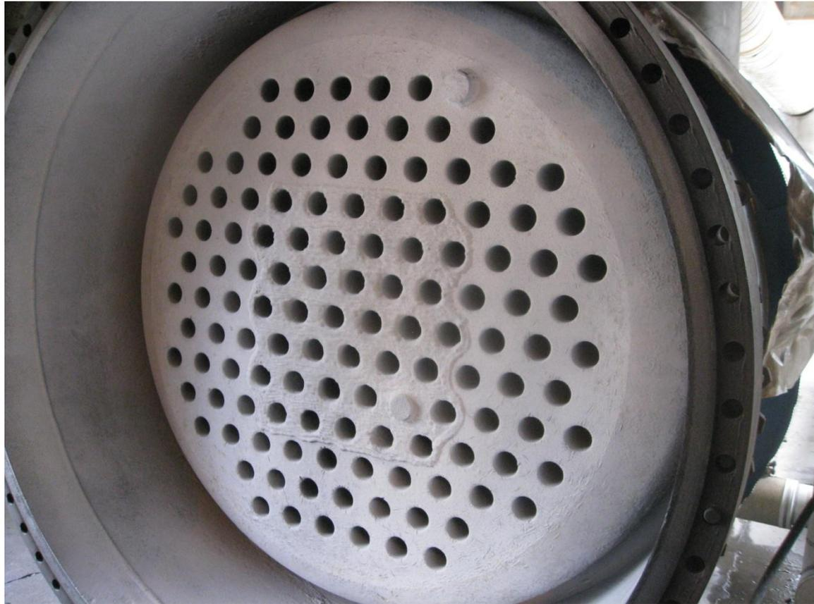
First coat dried at room temperature and ready for second coat.
